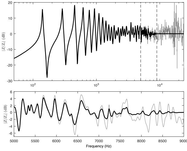
Figure 2: *Magnitude response of an alto saxophone impedance measurement (Bb3 fingering), normalized by the characteristic impedance of the input of the air column. Thin and thick curves are respectively used for raw and pre-processed data. Top: full band, with cross-fading region delimited by vertical lines. Bottom: cross-fading region.*
