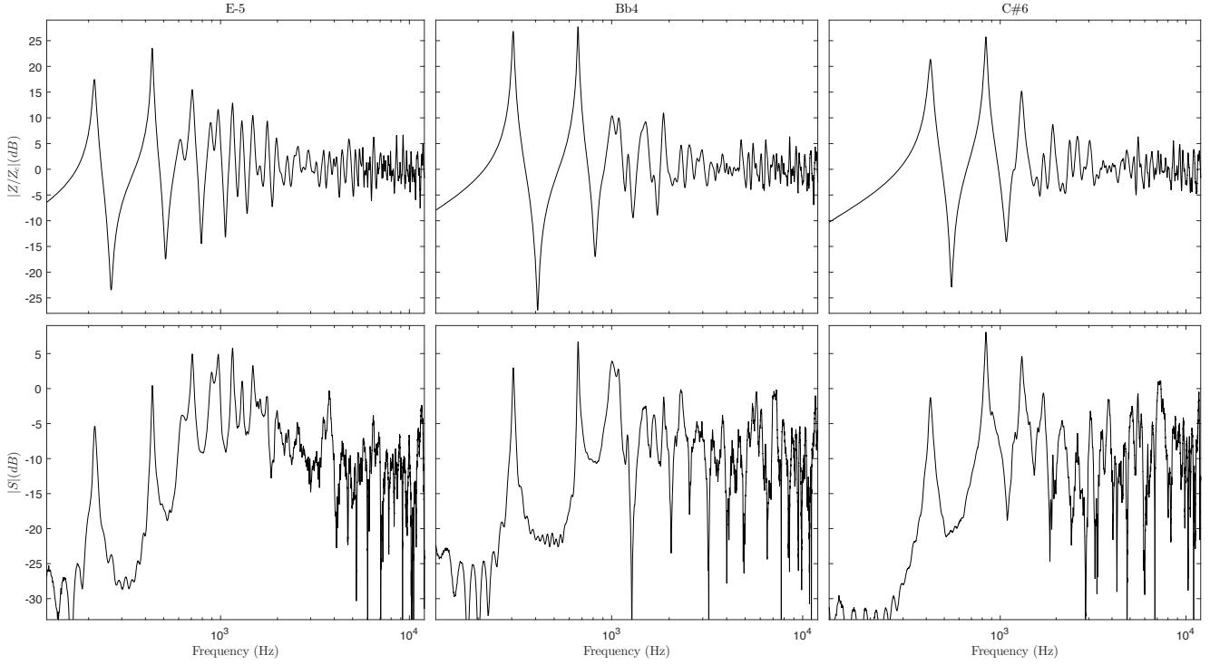
Figure 1: Magnitude response of impedance (top) and radiation (bottom) measurements for different fingering positions in an alto saxophone.
