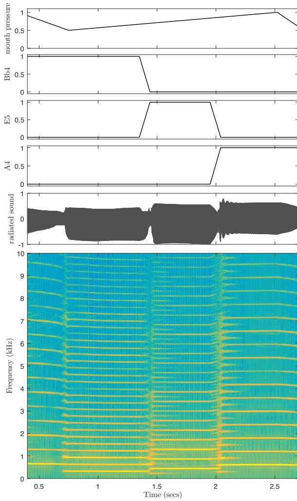
Figure 5: Sound synthesis example, with  $M = 32$  parallel sections per fingering. From top to bottom: mouth pressure (normalized units), weights  $w_f$  corresponding to Bb4, E-5, and A-4 fingerings, radiated sound pressure (normalized units), and a spectrogram of the radiated sound pressure.
