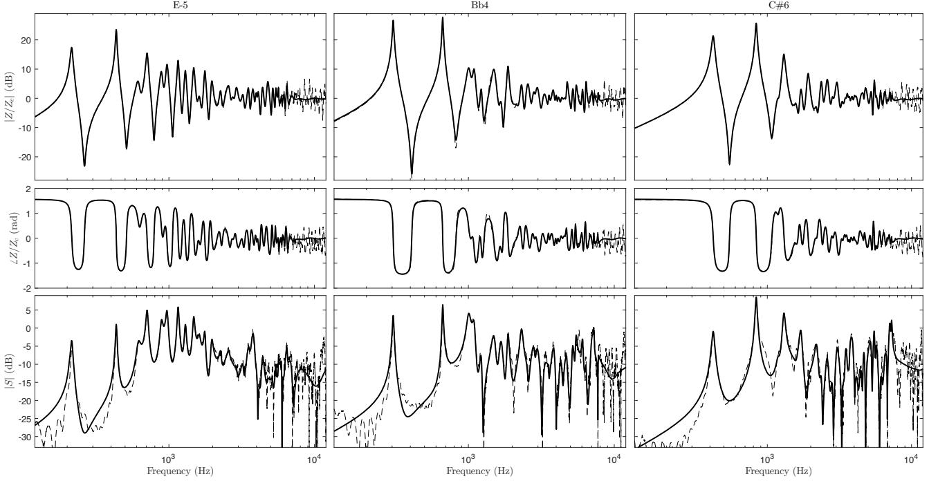
Figure 3: Example impedance and radiation models. All three fingerings were modeled with  $M = 32$  parallel sections each. From top to bottom: impedance magnitude response, impedance phase response, and radiation magnitude response. In each plot, dashed lines and thick lines are used to depict the measurement and the model respectively.
