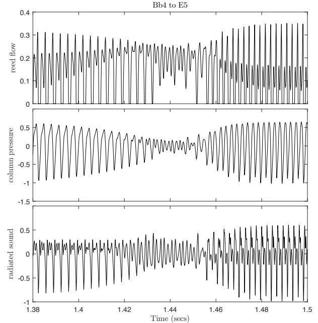
Figure 6: Detail of the transition between Bb4 to E5. From top to bottom, in normalized units: reed flow, air column input pressure, radiated sound pressure.
