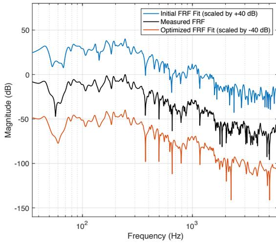
Figure 3: Microphone frequency response function (FRF) and fits with  $N = 88$  modes.
