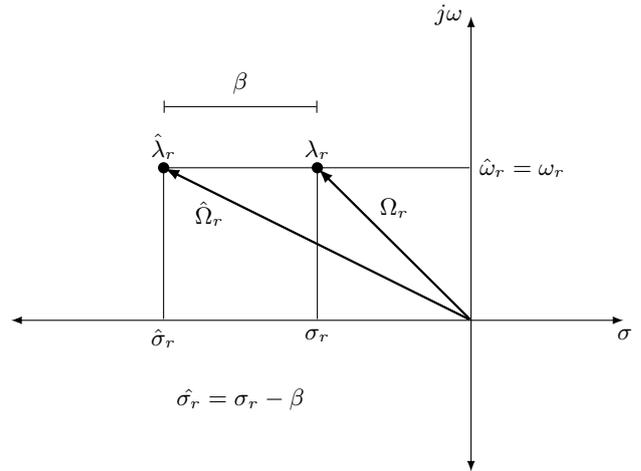
Figure 4: Effect of the exponential decay window in the complex plane.  $\beta$  is the exponential decay constant of the window.  $\lambda_r$ ,  $\omega_r$ ,  $\sigma_r$ , and  $\Omega_r$  are the eigenvalue, damped natural frequency, damping factor, and undamped natural frequency for mode  $r$ .  $\hat{\lambda}_r$ ,  $\hat{\omega}_r$ ,  $\hat{\sigma}_r$ , and  $\hat{\Omega}_r$  have the same meaning except for the windowed signal.
