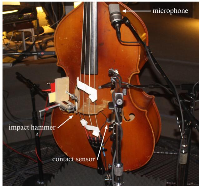
Figure 1: Measurement setup.
