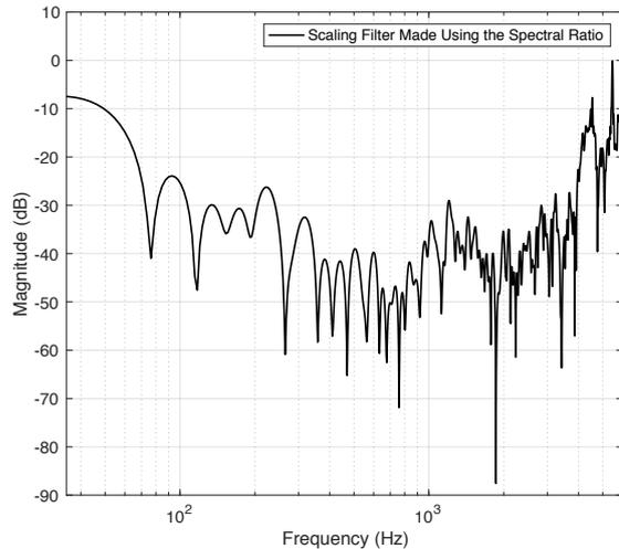
Figure 6: Spectral ratio scaling filter frequency response implemented using a 1200 tap FIR filter.
