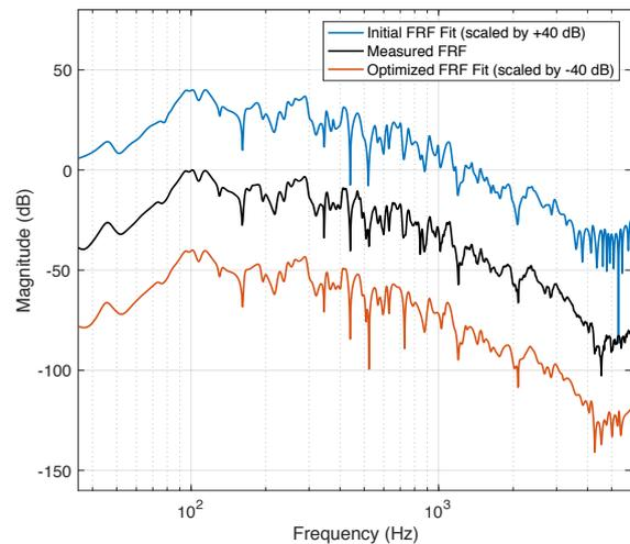
Figure 2: Contact sensor frequency response function (FRF) and fits with  $N = 88$  modes.
